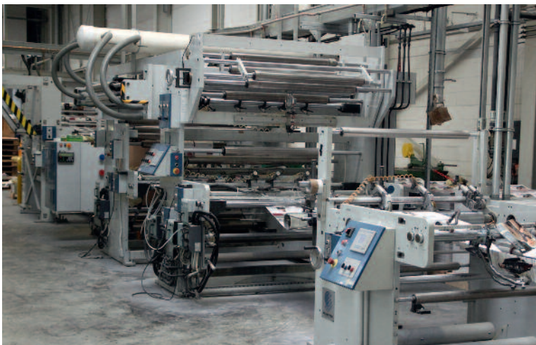
Left: The Scheffer finishing system is a key component for the production of unusual products. This is capable of die-cutting, perforating, gluing, lining or plough folding in a single pass.
