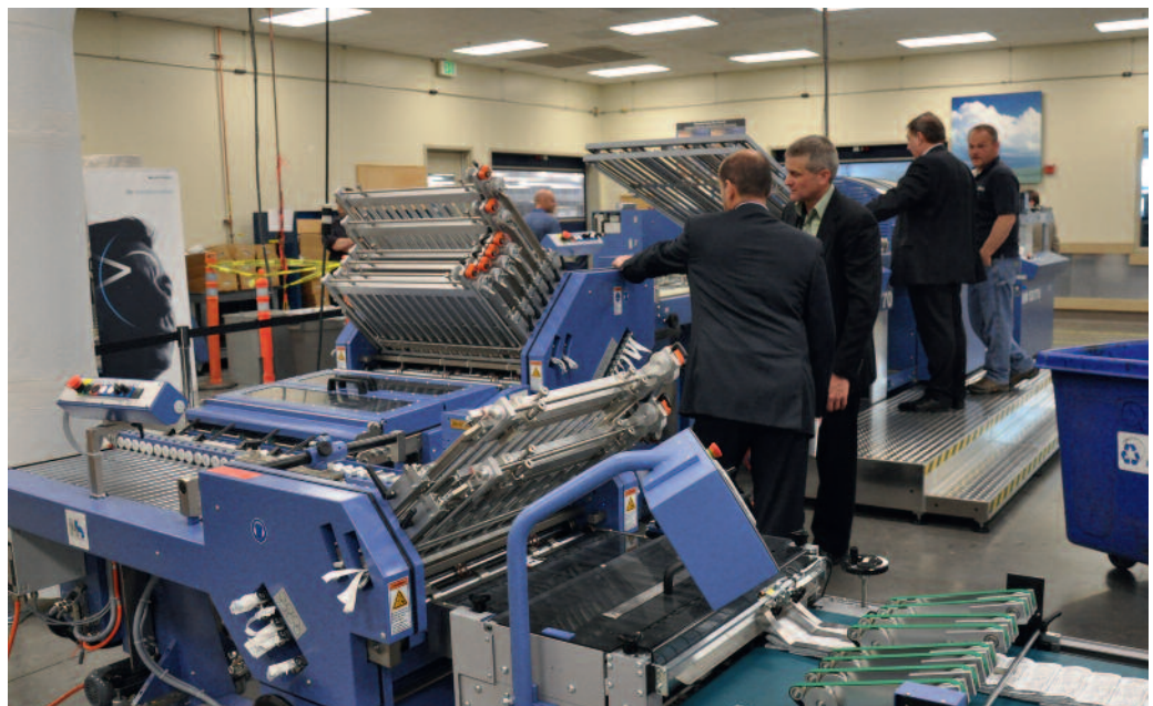
With up to ten folds, a specially designed MBO folder combined with an EM770 ejector module is required.
