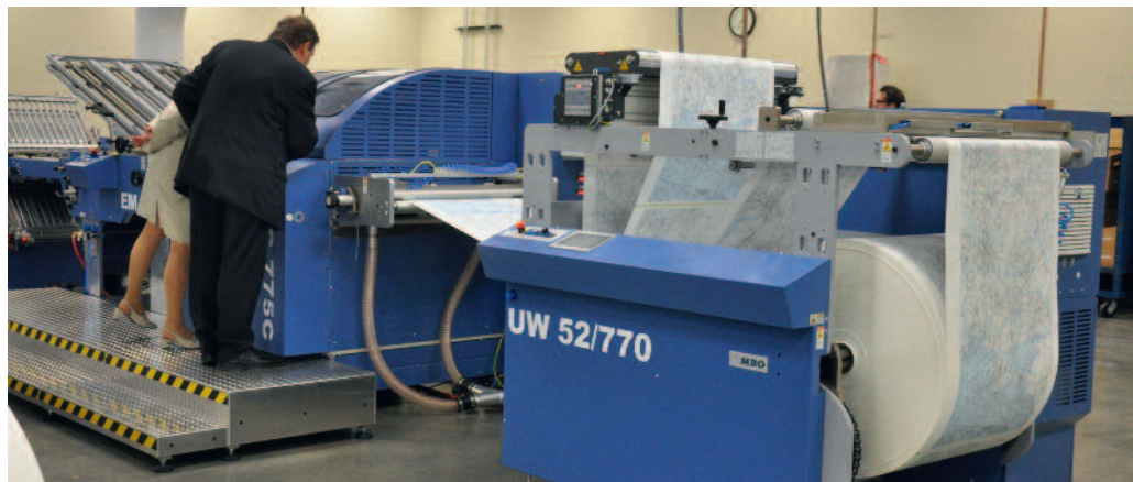
The printed reels are then unwound by a UW52/770 unwinder and fed into a sheeter and then a folder.
