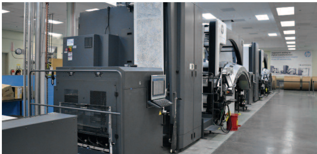
Aeronautical charts are reel-to-reel printed by an HP T300 reel-fed digital press at Jeppesen.
