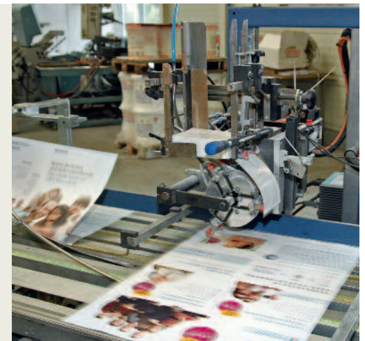
Left: The Scheffer finishing system is a key component for the production of unusual products. This is capable of die-cutting, perforating, gluing, lining or plough folding in a single pass.
